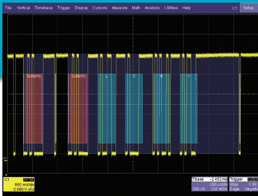
Color-coded overlaid protocol decode makes it easy to understand your serial data messages.
