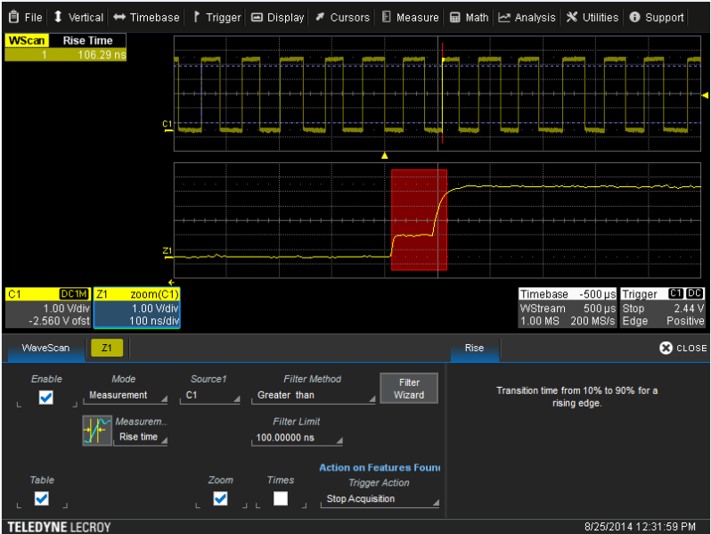
Figure 2: Here, WaveScan has found the glitch it was seeking in the input signal
