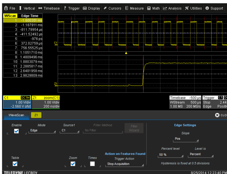
Figure 1: The initial setup screen for WaveScan is the starting point for deep signal exploration
